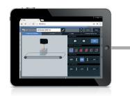
Multiple laser marking systems can be controlled from TCS+ running on a web browser. Each laser is represented in its own tab within the web browser. All laser systems need to be in the same network as the PC/browser-enabled device that is running TCS+ in a web browser. To control the laser systems through WiFi, each laser has to be equipped with a WiFi kit and logged into the customer's network.
